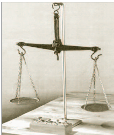
Fig. 1: Equal-arm beam balance, around 7000 BC
