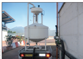
Master meter used for the verification of bottom loading road tankers in Naples
