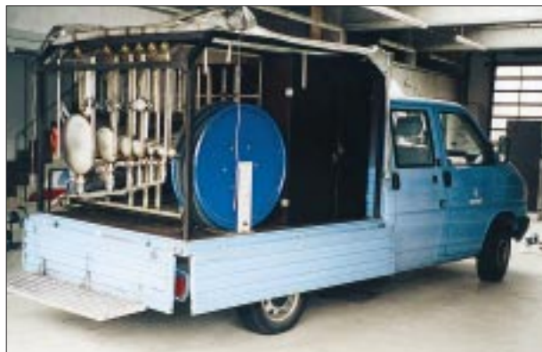
Fig. 1 Built-in testing facility in a car. While filling, the verification officer stands on the grating which is fixed to the tailboard. There is no intermediate storage of the product to be measured.
